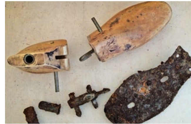
Shoe last parts (metal) and a dismantled last showing internal parts.
